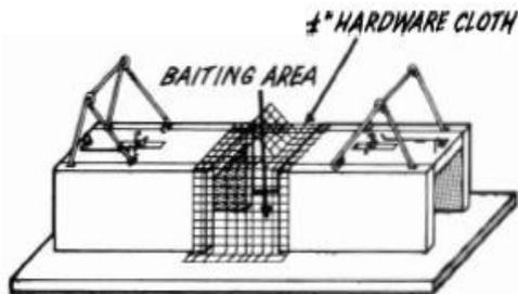
Two modified traps may also be placed back to back and secured to a board (1" × 4" × 18"). A small strip of hardware cloth connects the two and forms a baiting area. Baiting is accomplished by placing a handful of bait through a small door cut in the wire or through the open end of the trap.
