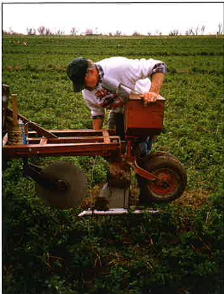
A burrow builder creates an artificial burrow and drops in the bait.
